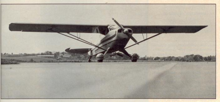
Spoilers, gull-wing doors and a large wing area make this homebuilt a natural for short fields, floats and load hauling. As a floatplane, gross weight is 2,200 pounds.
